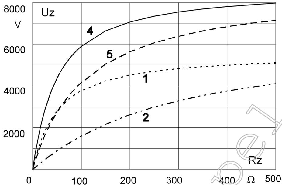
FIGURE 1. Dependence of the earthing voltage on a  $U_z$  post on its earthing resistance  $R_z$ . The curves are denoted according to the table 1.
